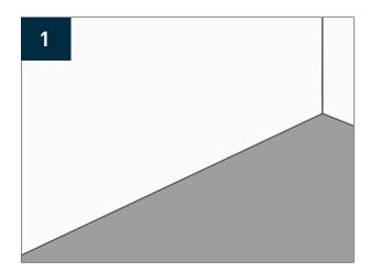
The panels must be installed onto a clean, solid surface, e.g. brick, rendered brick, fibrous cement sheeting or plywood. It can also be installed onto gyprock, if it has been secured correctly.
