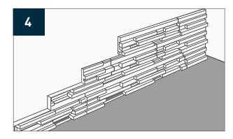
4. Start to lay Panels in a staggered brick like form leaving a 8mm gap at the top of the wall for an expansion gap.
