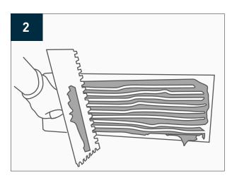
2. Adhesive must be applied to the back of each Panel with an 8mm notched trowel and then placed on the wall. Each panel when laid should be tapped into place so the adhesives take hold.
