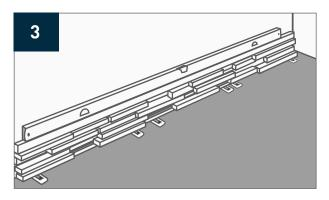
3. If proceeding with a horizontal application, set the first layer of Panels with a level sitting on 5mm packers to allow for an expansion gap.
