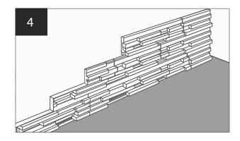
4. Start to lay Panels in a staggered brick like form leaving a 8mm gap at the top of the wall for an expansion gap.
